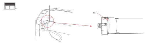
2 Adjusting the 'up position' end stop (shutter completely open):
