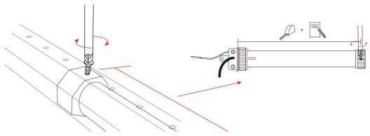
**4** Attach the retaining bracket on the appropriate side of the housing.
