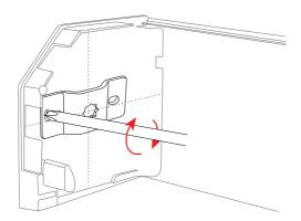
**5** Attach the roller with the motor installed in the housing, slotting the bracket into the retaining head (see diagram).
