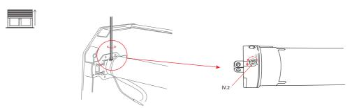
We recommend that you adjust the end stops gradually by only turning the adjustment screws a few turns at a time. Warning, depending on the size of your shutter, you may have to turn the screws several dozen times to get the correct setting.
