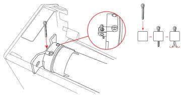
**7** Refit the shutter onto the roller in accordance with the instructions for your shutter or blind, taking care that the power cable or antenna does not impede it from rolling up.
