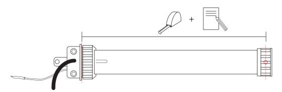
2 Insert the motor into the shutter roller, taking care to align the octagonal ring mark with the adjustment line located on the head of the motor. Only the head of the motor may extend beyond the roller.
