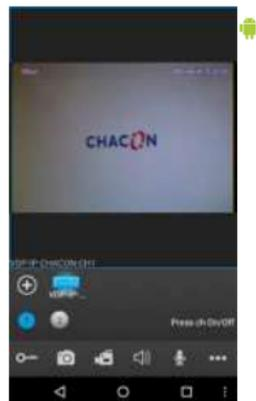
For all other mobile equipment's, that you want to add your IP VDP, please press the "+" button and select the option "Add a device that is connected to the internet". Select the option "Scan Qr Code" and scan the Qr Code that is in the back of the Unit.
