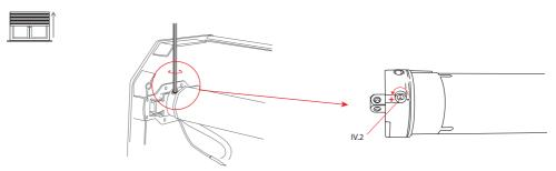
We recommend that you adjust the end stops gradually by only turning the adjustment screws a few turns at a time. Warning, depending on the size of your shutter, you may have to turn the screws several dozen times to get the correct setting.
