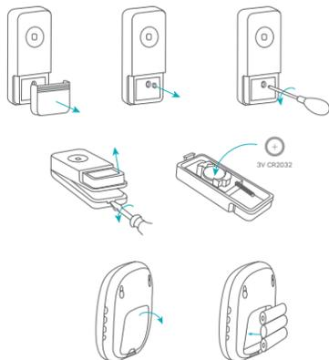
**1.2. Installing the battery (chime)**
