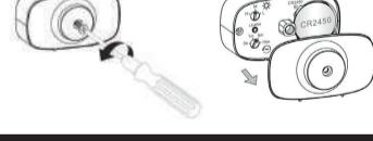
Open the back of the sensor with a crosshead screwdriver and remove the battery tab.
