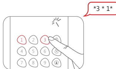
When one beep is heard and the LED indicator keeps on for 10 seconds, the setup is successful.
