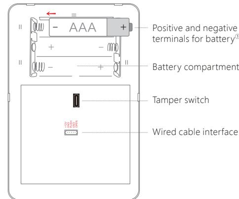
① The keypad beeps twice every two seconds and the LED indicator flashes once in case of low battery.
