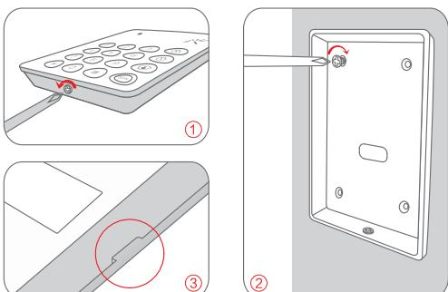
**Note:** Opening the rear cover of keypad will trigger tamper switch, please disarm the alarm by following the disarm instruction in page 21-22.
