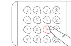
When one beep is heard and the LED indicator keeps on for 10 seconds, the setup is successful.
