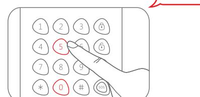
When one beep is heard and the LED indicator keeps on for 10 seconds, the setup is successful.
