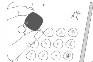
To clear the connection of RFID tags, input [admin code] + [#] to wake up the keypad and then press down [9] for six seconds. RFID tags are all cleared after one beep..
