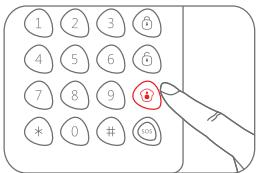
When the alarm panel receives the signal, the siren will beep once and the [Stay Mode] indicator will light on, the alarm system enters stay mode state.
