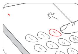
Under setup state, if there is no operation within 10 seconds, the keypad will exit setup state automatically. You can also press [#] to exit.
