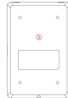
**Note:** Open the rear cover of keypad will trigger tamper switch, please dismiss the alarm by following the disarm instruction on page 21-22.
